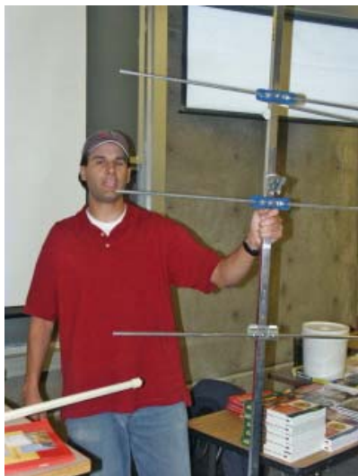
Chris Perri, KE7FYP, shows a collapsible, 5-element, two-meter Yagi. The design, from one of the ARRL publications, uses a modified FM broadcast antenna available from Radio Shack.
