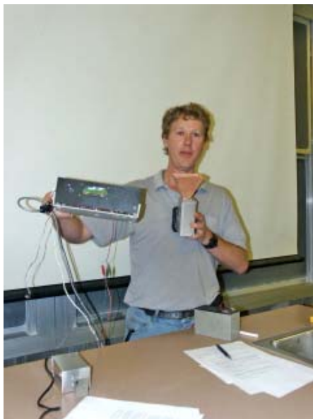
Clint Turner, KA7OEI, shows his unit to control Gunnplexer units on the 10- and 24-GHz bands. His box is unique because it measures temperature and makes adjustments to the tuning voltage to compensate for the Gunnplexer's normal frequency change with temperature. This improves frequency stability by a factor of 10-to-1 over using a fixed voltage. The controller can be pre-programmed with information about the temperature curves of several different Gunnplexers.
