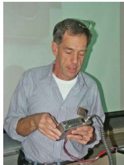
Dale Heisler, WJ7L, built a sequencer to solve a problem unique to mast-mounted preamplifiers. A preamp at the antenna solves the problem of degraded receive performance due to coax loss. A pitfall, however, is that transmitting while the preamp is still connected can destroy the preamp. The sequencer makes sure that components of the station go on and off in the right sequence during the switch from receive to transmit.
