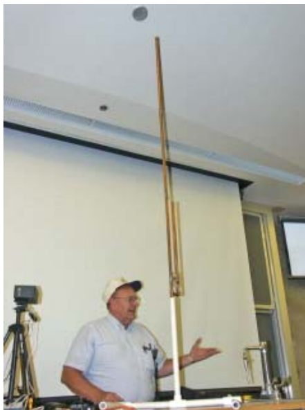
"Woody" Woodruff, KC7YLH, built a collapsible two-meter J-pole with a PVC base support. The J-pole is made of copper pipe sections held together with bungee cord as per a QST article. Woody says the antenna can be set up in a driveway in a very few minutes, and is useful for attracting questions from the public as well as providing a quick antenna for emergency situations.
