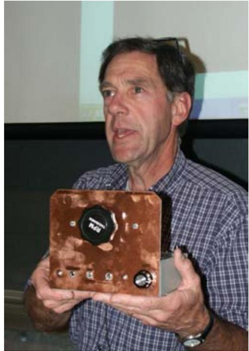
Dale Heisler, WJ7L, displays a homebrew 40-meter receiver with quadrature audio channels.
